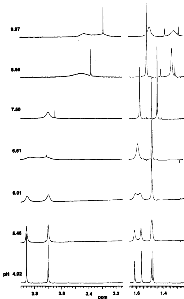
Figure 1. The methine (3.1–3.9 ppm) and methyl (1.25–1.65 ppm) regions of the 1 H NMR spectra of aqueous solutions containing 0.010 M PSH, 0.005 M PSSeSP, and 0.3 M KCl at 25 °C. The two regions are plotted with different vertical scales. The assignment of resonances in the pH 4.02 spectrum is as follows: 3.860 ppm, methine proton of PSSeSP; 3.699 ppm, methine proton of PSH; 1.614 and 1.491 ppm, methyl protons of PSSeSP; 1.564 and 1.479 ppm, methyl protons of PSH. The additional, sharp resonances which are present in spectra at pH 6.01 and higher are due to PSSP, as discussed in the text.
